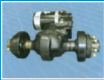
Advanced transverse transmission system
